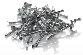
afterwards Chip generation with high frequency turning
