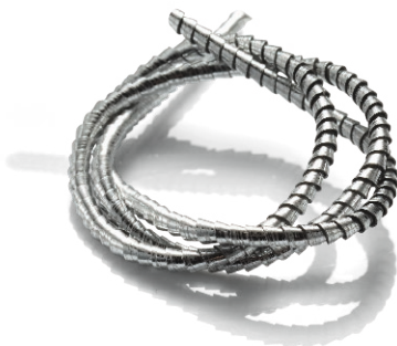
Chip formation with conventional machining
