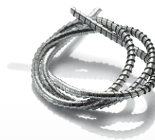
before Chip generation with conventional machining
